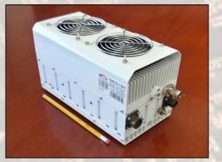
This smallest and lightest 100W L-To C-Band Block Up Converter is based on GaN technology.Incomparable low power consumption, double L.O., Field- Exchangeable connector and auto-ranging (80-240 VAC) powering features make unit universal for any C-Band application. M&C (FSK) capability enables troubleshooting, monitoring and controlling the BUC. The user can choose internal 10MHz high stability reference if the corresponding modulator does notprovide it.
