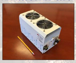
This is a unique Ext. C-Band (5.850-6.725 GHz) 100W Block Up Converter powered with auto-ranging 80-240 VAC unit, designed for mobile applications especially when an earth station needs to be able to use different C-Band (Standard or Palapa) transponders or satellites. It's light enough to be mounted on a feed horn of most antennas.
