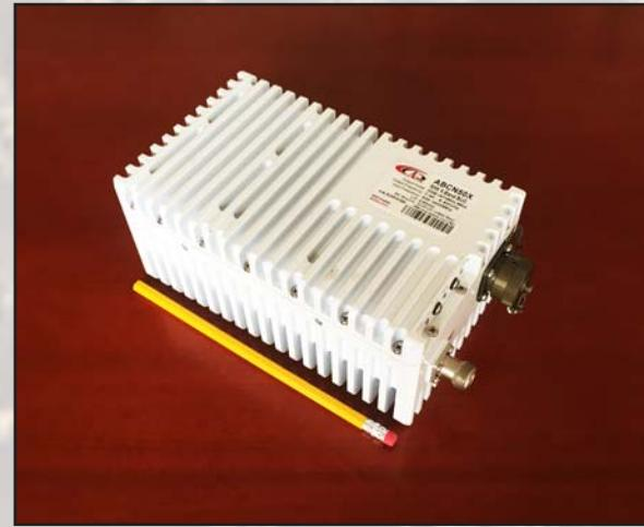
This smallest and lightest 50W(min) L-To X-Band Block Up Converter is based on GaN technology. It could be mounted directly on a feed horn. High power efficiency resulting in low current (<3.9 amps).
