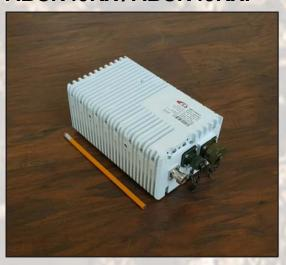
This smallest and lightest 40W L-To Ku-Band Block Up Converter is designed to be mounted on a feed horn. The unit is ideal for portable and mobile applications. Double – L.O. feature makes unit universal for Ku-Band requirements. DC powered through the MS Connector and consumes less than 195W.
