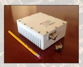
This smallest and lightest 7W L-To Ku-Band Block Up Converter is based on GaN technology. Double L.O. and field- Exchangeable connector make unit universal for any Ku-Band application. Incomparable low power consumption allowes the BUC to be powered by iDirect and similar modems. Internal 10MHz reference option enables using the BUC with the modems without 10MHz reference.
