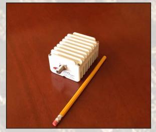
This smallest and lightest 6W L-To Ku-Band Block Up Converter is based on GaN technology and is designed to be mounted directly on the feed horn. High power efficiency resulting in low current (< 1 amps) consumption allows to use this BUC with any modem without an external power supply.
