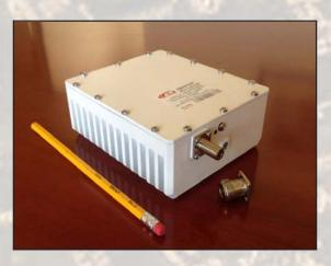
This smallest and lightest 6W L-To Low Ku-Band Block Up Converter is based on GaN technology. Double L.O. and field- Exchangeable connector make unit universal for any Ku-Band application. Incomparable low power consumption allowes the BUC to be powered by iDirect and similar modems. Internal 10MHz reference option enables using the BUC with the modems without 10MHz reference.
