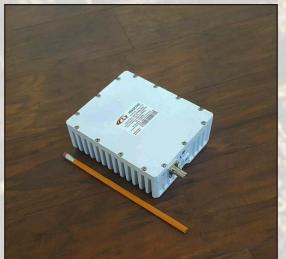
This smallest and lightest 6W L-To Ext. (13.75-14.50GHz) Ku-Band Block Up Converter is based on GaN technology. Incomparable low power consumption allowes the BUC to be powered by iDirect and similar modems.
