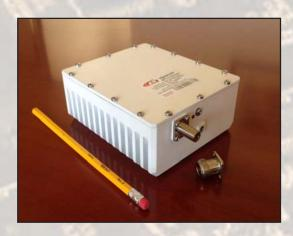
This smallest and lightest 6W L-To Ku-Band Block Up Converter is based on GaN technology. Double L.O. and field- Exchangeable connector make unit universal for any Ku-Band application. Incomparable low power consumption allowes the BUC to be powered by iDirect and similar modems. Internal 10MHz reference option enables using the BUC with the modems without 10MHz reference.
