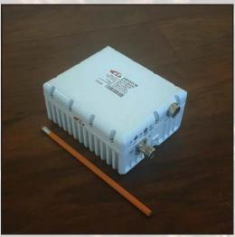
This smallest and lightest 5W L-To C-Band Block Up Converter is based on GaN technology. It is designed to be mounted on the feed horn. High power efficiency resulting in the low current (<=1 amps @ 24 VDC). The unit covers all three C-Band sub-bands: Standard (5.850-6.425 GHz), Palapa (6.365-6.725 GHz) and Insat (6.725-7.05 GHz).
