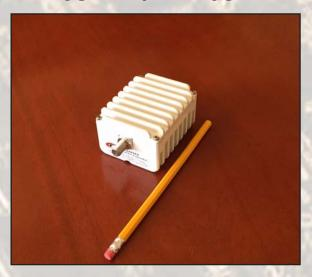
This smallest and lightest 5W L-To Low Ku-Band Block Up Converter is based on GaN technology and is designed to be mounted directly on the feed horn. High power efficiency resulting in low current (< 1 amps) consumption allows to use this BUC with any modem without an external power supply.
