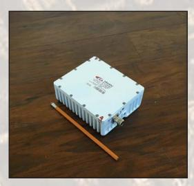
This smallest and lightest 5W L-To C-Band Block Up Converter is based on GaN technology. High power efficiency resulting in the lowest power consumption. The unit covers Standard (5.850-6.425 GHz) and Palapa (6.365-6.725 GHz) C-Band frequencies.
