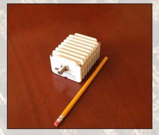
This smallest and lightest 4W L-To Low Ku-Band Block Up Converter is based on GaN technology and is designed to be mounted directly on the feed horn. High power efficiency resulting in low current (< 1 amps) consumption allows to use this BUC with any modem without an external power supply.
