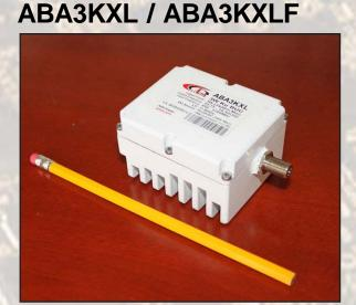
This smallest and lightest 3W L-To Ku-Band Block Up Converter is based on GaN technology and is designed to be mounted directly on the feed horn. High power efficiency resulting in low current (< 1 amps) consumption allows user to pass DC supply voltage via IF cable. The unit is ideal for network and point to point, data distribution, portable and emergency applications.
