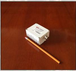
This smallest and lightest 3W L-To Ku-Band Block Up Converter is based on GaN technology and is designed to be mounted directly on the feed horn. High power efficiency resulting in low current (< 1 amps) consumption allows user to pass DC supply voltage via IF cable. The unit is ideal for network and point to point, data distribution, portable and emergency applications.
