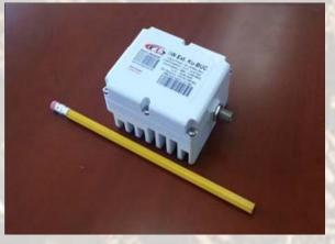
This smallest and lightest 2W L-To Ku-Band Block Up Converter is based on GaN technology and is designed to be mounted directly on the feed horn. High power efficiency resulting in low current (< 1 amps) consumption allows user to pass DC supply voltage via IF cable. The unit is ideal for network and point to point, data distribution, portable and emergency applications.
