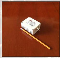
This smallest and lightest 2W L-To Ku-Band Block Up Converter is based on GaN technology and is designed to be mounted directly on the feed horn. High power efficiency resulting in low current (<1 amps) consumption allows user to pass DC supply voltage via IF cable. The unit is ideal for network and point to point, data distribution, portable and emergency applications.
