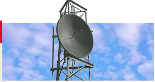
The reflector is constructed from 3.1 mm (0.125 in) thick aluminum fabricated to a surface accuracy of 0.5 mm (0.020 in) rms or better.
