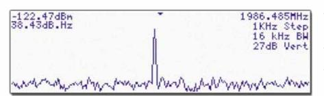
The Spectral Display offers a convenient amplitude vs. frequency display of the received signal. The display is useful for system fault isolation, for routine maintenance and is also cost effective when a full function spectrum analyzer is not available or necessary.
